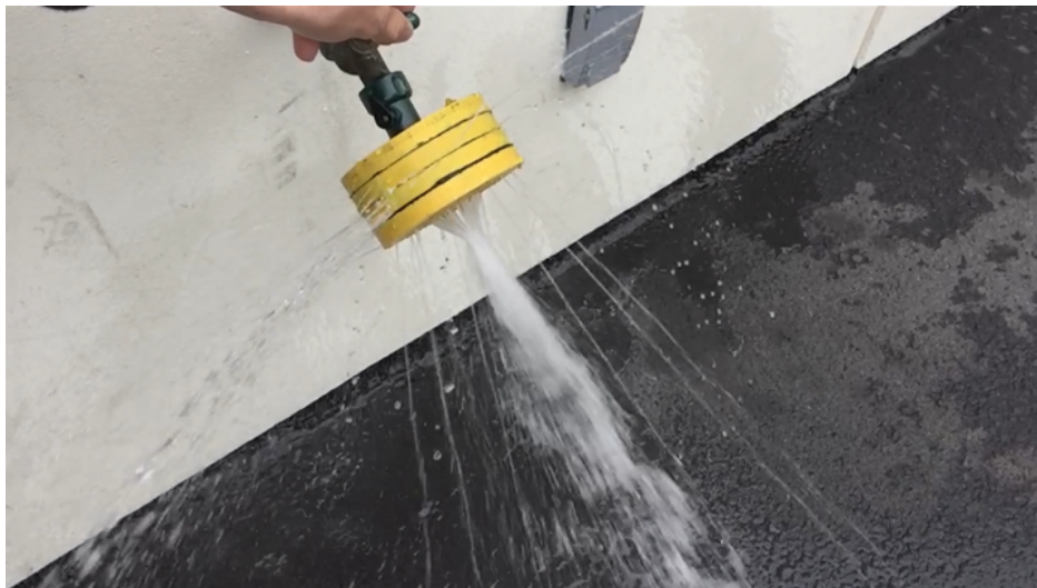
Figure 6: ABS-Injector Cold Flow Test
